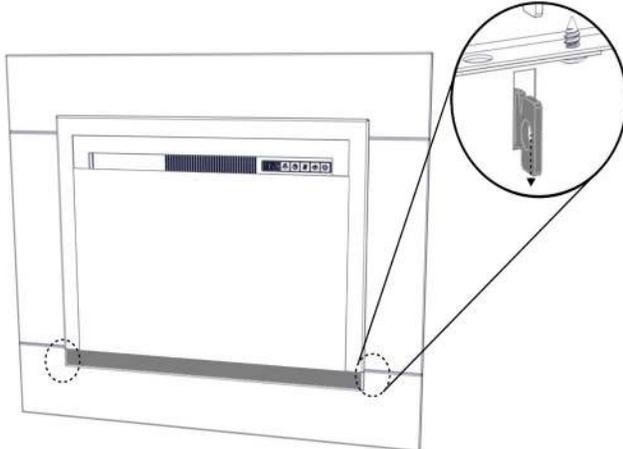
INSERT THE TWO BRACKETS INTO THE SLOTS ON THE BOTTOM
