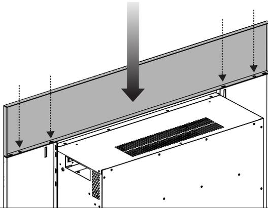
SECURE THE TOP TRIM USING FOUR SCREWS.
