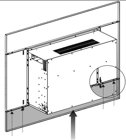
TIGHTEN TWO INTERIOR SCREWS AND SECURE BOTTOM TRIM USING
