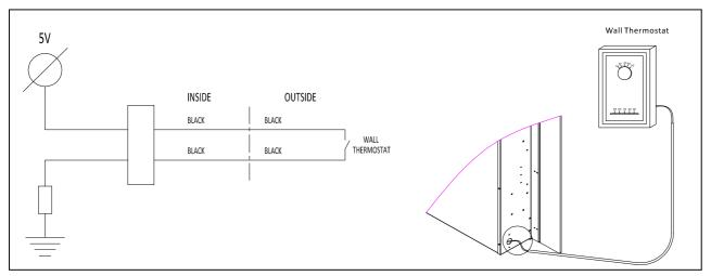
NOTE: THE WALL THERM OSTAT WILL WORK ONLY WHEN THE HEATER IS SET TO TEMP. SETTING PLEASE REFER TO THE M ANUAL CONTROL AND THE REM OTE CONTROL
