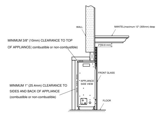
The fireplace insert may be placed within a framed enclosure that is level, dry, and capable of supporting the weight of the appliance and front glass. It may be placed directly on wood or a non-combustible surface (not on linoleum or carpet). The minimum clearance from the top of the appliance to a mantel (combustible or non-combustible) is 2" (50.8mm). The sides and back must maintain 1" (25.4mm) clearance to any material. The top must maintain a 3/8" (10mm) clearance to any material.
