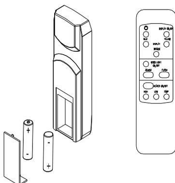
For remote to function make sure the heater is plugged in and main power switch located on the bottom left hand side is at position I.
